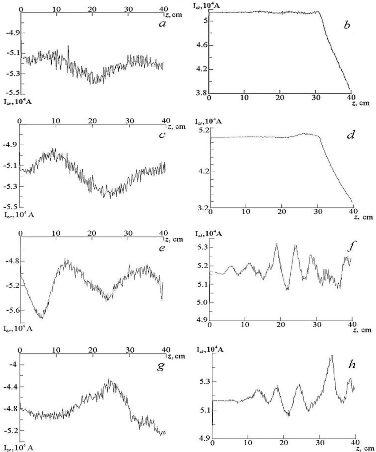
Fig. 3. The dependence of the electron beam (left column) and ion beam (right column) longitudinal current on the longitudinal coordinate  $z$  after  $2\tau$ . (a, b) – AE injection is absent; (c, d) – after  $0.5\tau$  from right side AE are injected during  $0.5\tau$ ; (e, f) – after  $\tau$  from right side AE are injected with velocity  $0.27c$ ; (g, h) – after  $\tau$  from right side AE are injected with velocity  $0.5c$
