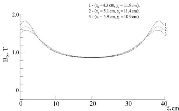
Fig. 2. The dependence of the external longitudinal magnetic field on the longitudinal coordinate  $z$  at different points  $x, y$
