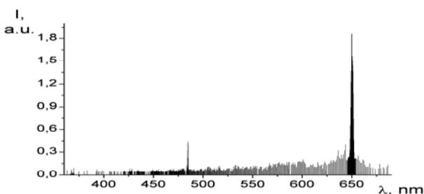
Fig. 3. The emission spectra of discharges in air at a pressure  $P = 4.8$  Pa
