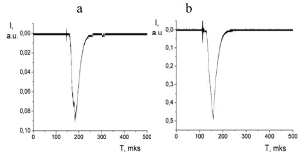
Fig. 4. Dependence of the optical radiation intensity on time for the wavelength 485 nm within a duration of one high-voltage pulse for gas pressures of  $P = 28$  (a) and 4.8 Pa (b)
