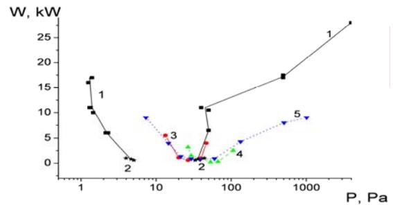
Fig. 1. Dependences for breakdown power of a microwave signals with a stochastically jumping phase versus a pressure for air in the optimal BPG mode (curves 1 – ■, 2 – \*), in the non-optimal BPG mode: for air (curve 3 – ●), argon (curve 4 – ▲), helium (curve 5 – ▼), respectively, at narrowband signal
