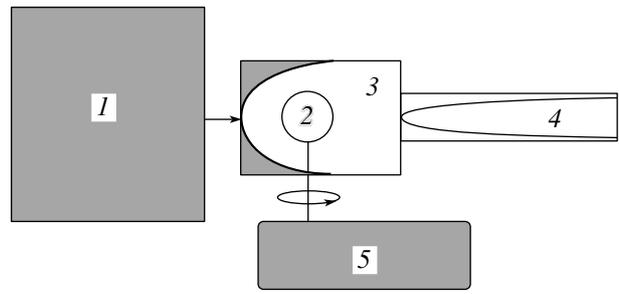
**Fig. 14.** Block diagram of a microwave-discharge-based light source: (1) power supply unit, high-power microwave generator, and matching system; (2) quartz shell filled with an Ar-S gas mixture; (3) microwave cavity and light output system; (4) lightguides; and (5) system for rotation and forced cooling of the quartz shell.
