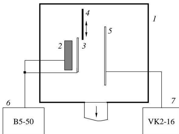
**Fig. 1.** Schematic of the experimental device: (1) vacuum chamber, (2)  $\text{Pu}^{239}$  radioisotope source of  $\alpha$ -particles, (3) target, (4) movable diaphragm, (5) collector, (6) B5-50 dc source, and (7) electrometric voltmeter.
