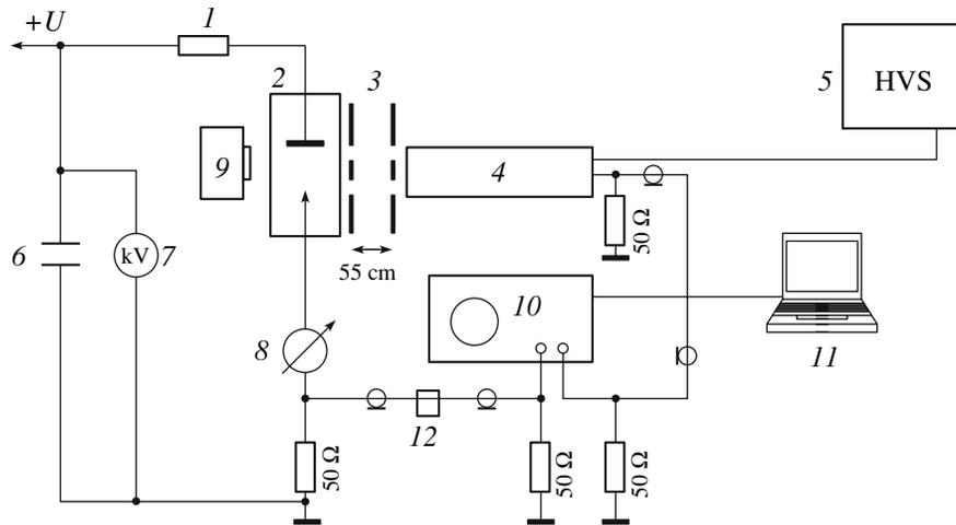
**Fig. 1.** Block diagram of the experimental setup: (1) 130-k $\Omega$  ballast resistor, (2) discharge cell, (3) slit, (4) FEU-36 photomultiplier, (5) photomultiplier high-voltage supply, (6) 2200-pF voltage filtering capacitor, (7) S196 kilovoltmeter, (8) M906 microammeter; (9) Olympus C7070 camera, (10) Tektronix TDS210 oscilloscope, (11) IBM PC, and (12) 38-ns delay line.
