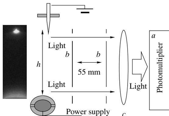
**Fig. 2.** Photograph of a negative corona and simplified optical scheme of the experiment: (*h*) discharge gap, (*a*) photocathode of the FEU-36 photomultiplier, (*b*) slits, and (*c*) quartz lens.
