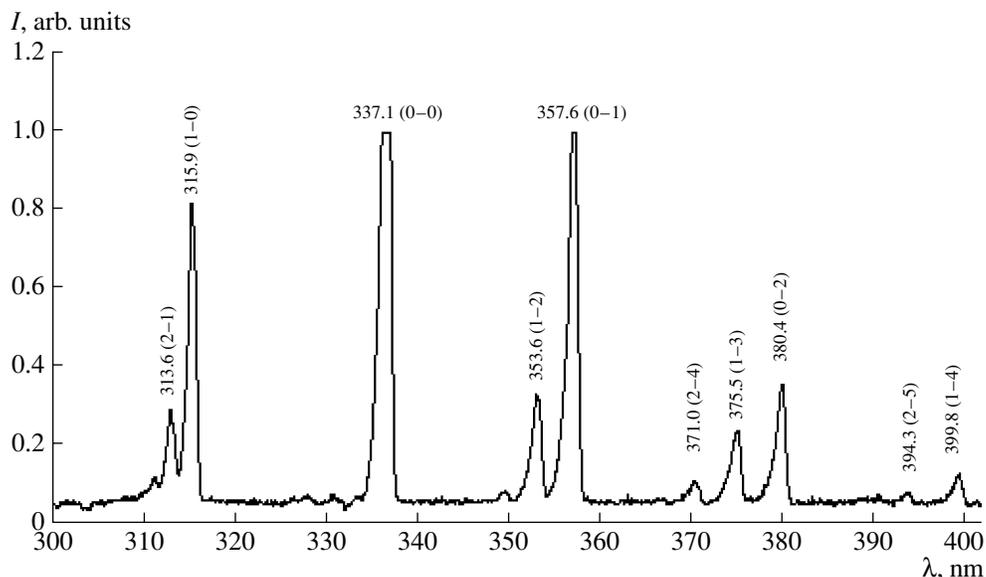
**Fig. 6.** Emission spectrum from the cathode region of a negative air corona operating in the Trichel-pulse mode in the point-to-sphere electrode geometry. The gap length is  $d = 15 \text{ mm}$ , the voltage is  $17 \text{ kV}$ , and the pulse repetition period is  $T = 2.5 \mu\text{s}$ .
