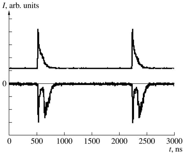
**Fig. 3.** Typical waveforms of the discharge current (upper curve) and the synchronized photomultiplier signal (lower curve) for a negative corona operating in the Trichel-pulse mode. The gap length is 7 mm,  $U = 9.6$  kV, and  $I_{av} = 34$   $\mu$ A.
