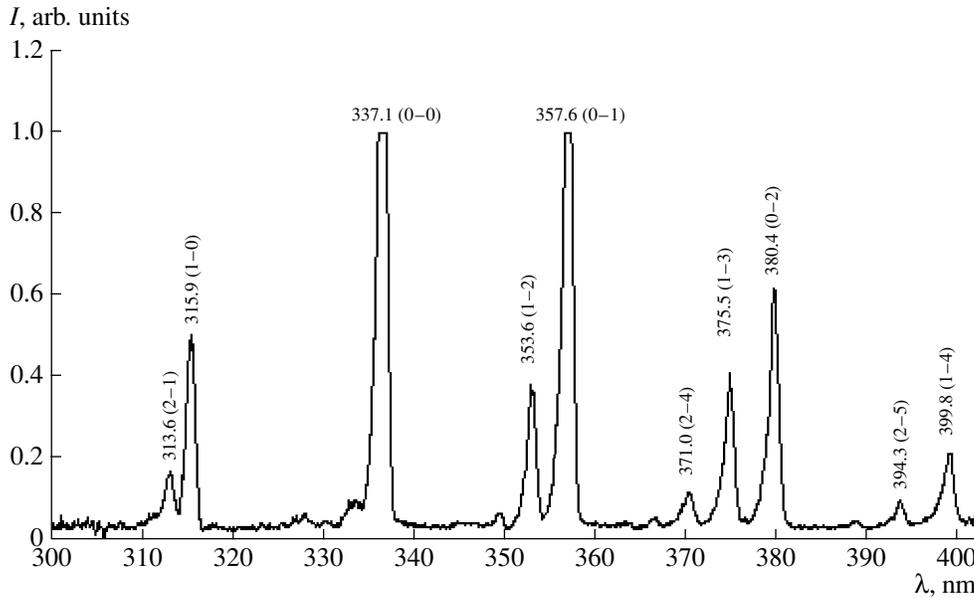
**Fig. 7.** Emission spectrum from the anode region of a negative air corona operating in the Trichel-pulse mode in the point-to-sphere electrode geometry. The gap length is  $d = 15$  mm, the voltage is 17 kV, and the pulse repetition period is  $T = 2.5$   $\mu$ s.
